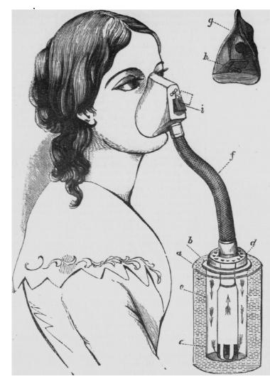
Perpendicular Section of Inhaler, on a scale of one-half the dimensions.
