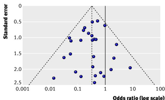
**Fig 1** Example of symmetrical funnel plot. The outer dashed lines indicate the triangular region within which 95% of studies are expected to lie in the absence of both biases and heterogeneity (fixed effect summary log odds ratio  $\pm 1.96 \times$  standard error of summary log odds ratio). The solid vertical line corresponds to no intervention effect
