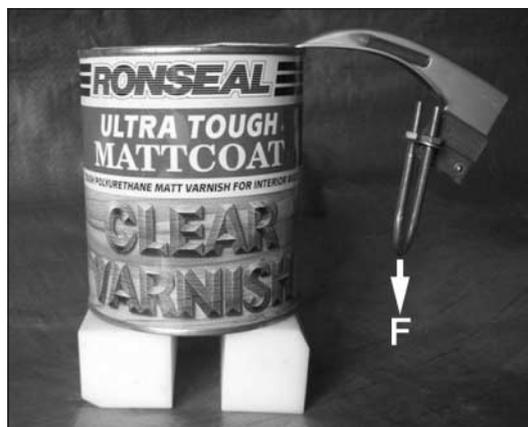
Fig 1 The force needed to open each tin was applied in direction F
