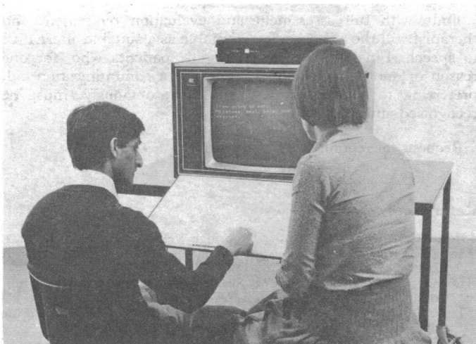
SPLINK consisting of communication board, microprocessor, and domestic television set.
