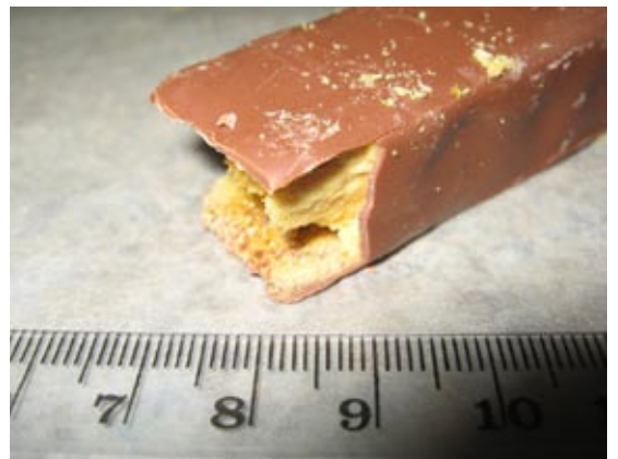
Fig 5 | “Blow-out” fracture at higher fall heights in Crunchie chocolate bar
