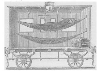
in the railway-van is for young and active persons, as an educated agility is necessary for entering one of these hammocks suspended four feet from the ground. The elastic cord on each side of the upper hammock moderates lateral swing when the carriage is running fast. The lower hammock is for the aged and infirm. This mode of travelling continues to give great satisfaction to invalids; and we recommend any tourist to provide himself with one of these portable accessories.
