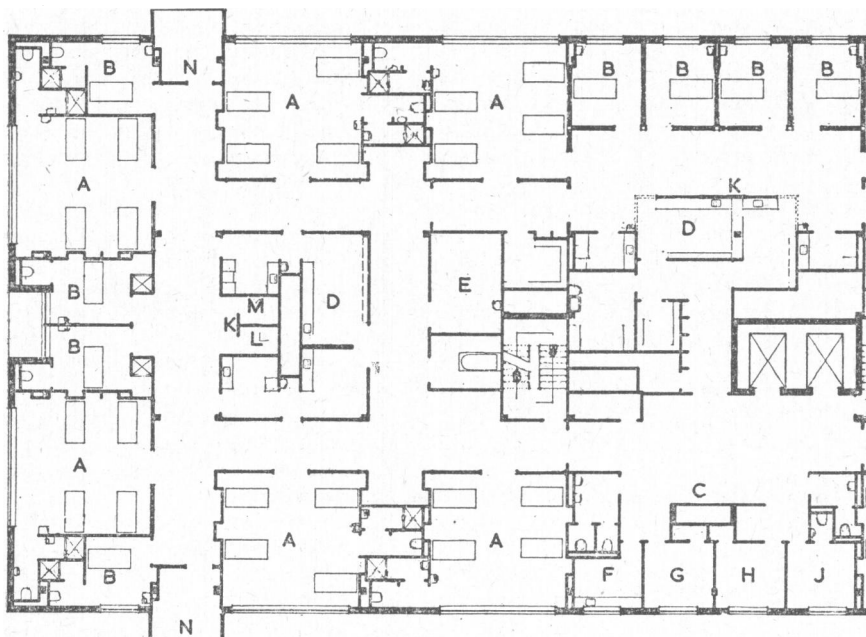
A.—4-bed wards. B.—Single bed wards. C.—Reception. D.—Preparation. E.—Treatment. F.—Laboratory. G.—Consultant. H.—Administrative sister. J.—Interview. K.—Nurses' station. L.—Sister. M.—House officer. N.—Day space.
