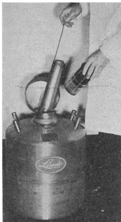
FIG. 1.—Refrigerator. One of the six canisters being removed.
