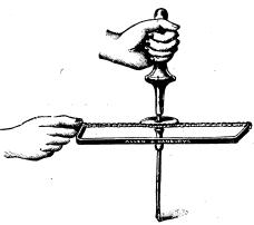
The drill is fitted into a chuck con-nected to a toothed wheel which is rotated by a chain stretched on a bow. The great advantage of the instrument consists in the ease with which even the hardest bone can be drilled with
