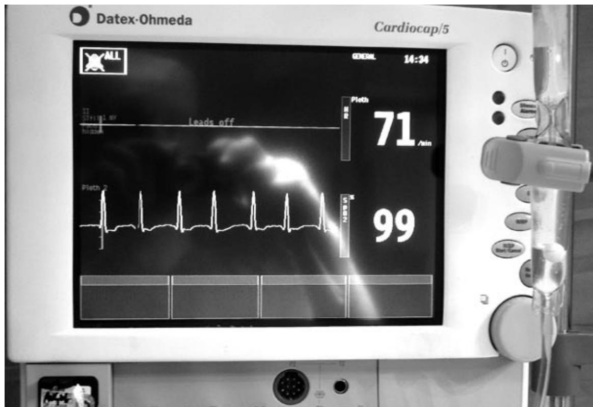
An oxygen saturation probe attached to a drip chamber produced what looked like an ECG and reassuringly normal oxygen saturations
