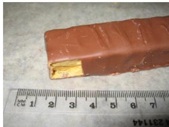
Fig 4 | Splinter fracture in Crunchie chocolate bar
