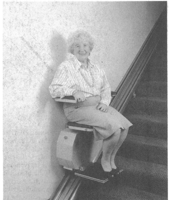
Stairlifts sit on a guiding rail, which is superficially mounted on to the staircase itself. They are as compact as possible, folding up to take about 25 cm of the stair width. The seat and footplate each fold, sometimes together, other times independently. The arms may fold up and, if so, will usually have a safety mechanism to prevent the stairlift from moving when the arm is upright. Sometimes the seat swivels (with a handle release mechanism) so that access on and off the seat can be made easier at the top and bottom of the stairs, where space may be limited. In case of a power failure or breakdown there is a hand wind facility to lower the stairlift down the staircase
