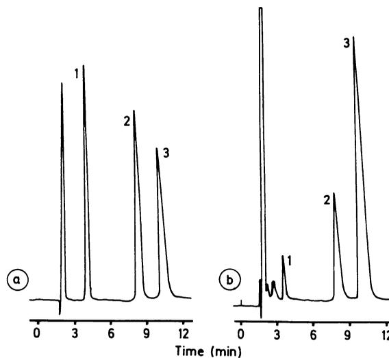
FIG 2—Separation by high performance liquid chromatography of deuterioporphyrin (1), mesoporphyrin (2), and protoporphyrin (3). (a) Standard mixture. (b) Yeast tablet extract. Column: SAS-Hypersil ( $15 \text{ cm} \times 5 \text{ mm}$ ); eluent;  $65\%$  (vol/vol) methanol in  $1.0 \text{ M}$  ammonium acetate; flow rate:  $1 \text{ ml/min}$ ; fluorescence detector: excitation  $404 \text{ nm}$ , emission  $618 \text{ nm}$ .
