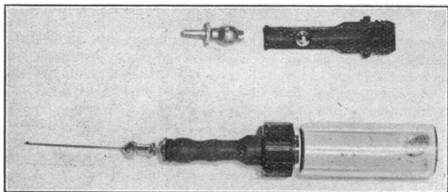
from the autoclave it is pushed down over the bulge in the rubber tube to form a sterile airtight fitting. Before use inspect the unit to see that the portion of the tube below the ball-bearing is collapsed, indicating a vacuum.
