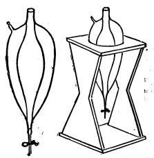
be controlled by a clip on the tubing attached to its exit. The flask is kept kept flask sterile by being filled with alcohol when not in use. The apparatus is adaptable for any purpose in which it is necessary to introduce warm fluids into the body via the veins, tissues, or rectum. I have found it extremely valuable in the treatment of shock during or after surgical
